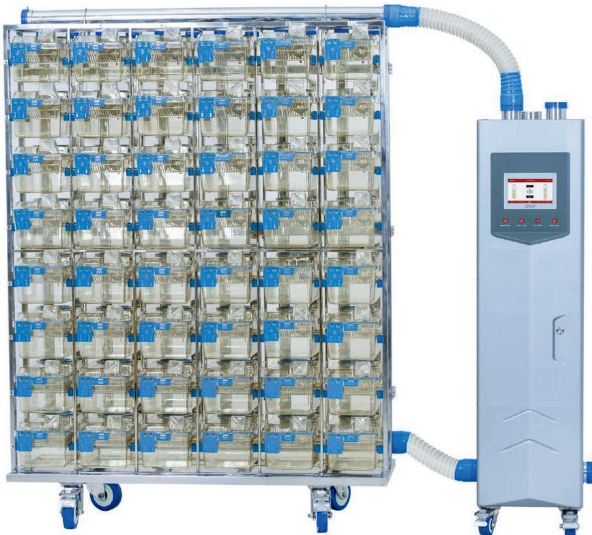
**Ventilator unit fitted with inbuilt UV-C light inside the cabinet for disinfection of the exhaust air coming from cages before releasing to the external environment.\***
